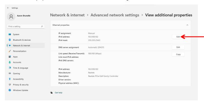
10. Click the drop-down and switch back to "Automatic (DHCP)". Then press the Save button to exit. Then click on "Advanced network settings".
