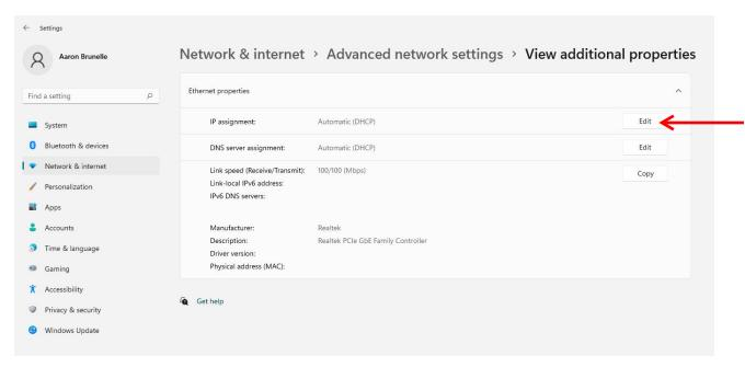
6. Click the drop-down and select "Manual". Then switch IPv4 to "On". Then, for the IP address take the IP address on the controller and increment/decriment it by 1 (i.e. if the controller IP address is 10.0.100.101, use 10.0.100.102 or 10.0.100.100). For the Subnet mask match the Subnet mask on the controller. Leave all other settings alone. Then press the Save button to exit. Then click on "Advanced network settings".
